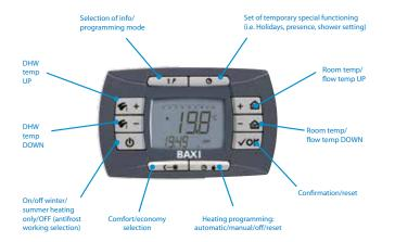
Luna3 Comfort models feature a removable control panel/thermostat that enables remote programming of the heating system, domestic hot water adjustment and full boiler diagnostics.
