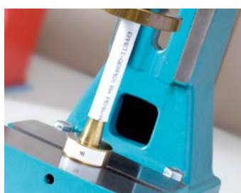
Enlargement Test Test performed both in production and in the laboratory to verify the quality of welds and the adhesion of individual layers.
