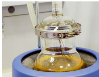
Verify degree of bonding (cross-linking) Verification performed in the laboratory to check the correct level (%) of cross-linking.
