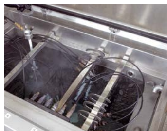
Resistance to internal pressure Test resistance to a specific internal pressure at 95 °C; the pressure value is chosen as a function of the type of pipe (maximum diameter, aluminium thickness) and the duration of the test (22h, 165h, 1000h), by referring to the relative regression curves.
