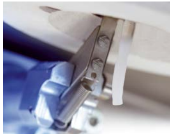
Melt Flow Index (MFI) Verify compliance of the polymer raw materials to be used.
