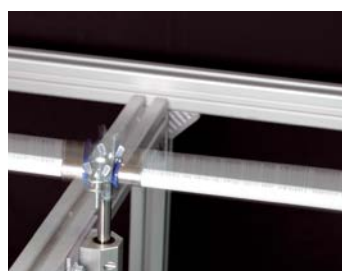
Vibration test Vibration test on a system consisting of the pipe and fittings which is subjected to 330 alternating bending cycles with an internal pressure of 15 bar at room temperature.
